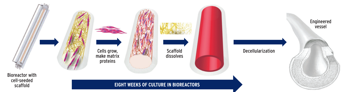
FIGURE 1 | Humacyte process for generating universally implantable regenerative human acellular vessel
