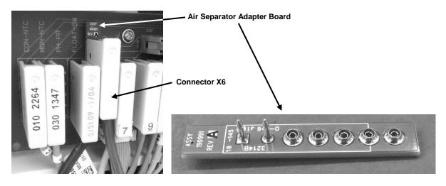
Replacement or spare Air Separator Adapter Boards are available by ordering the Air Separator Adapter Board Kit (P/N 191011). The kit includes an Air Separator Adapter Board and installation instructions.
