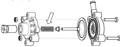
Part number **M50328** is now available for a complete Loading Pressure Regulator with the stronger spring already installed. This new part eliminates the need to replace the spring.
